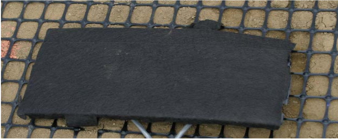
Figure 3.13. Geogrid strain gage protection, strip drain (Howard 2006).
