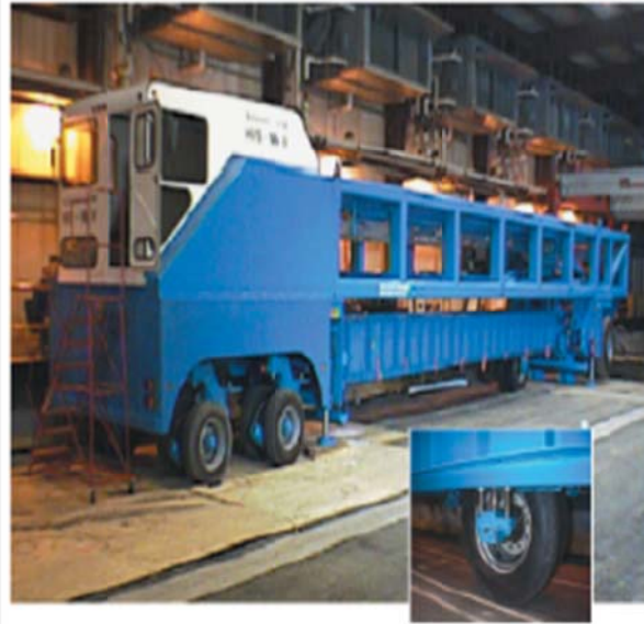
Figure 2.2. Heavy Vehicle Simulator (HVS) (Perkins and Cortez 2005).
