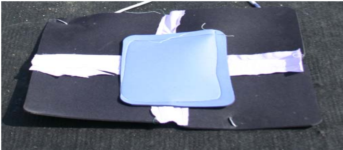
Figure 3.14. Geotextile strain gage protection, neoprene pad (Howard 2006).
